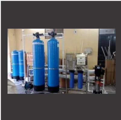
1000LPH Industrial RO System Plant
